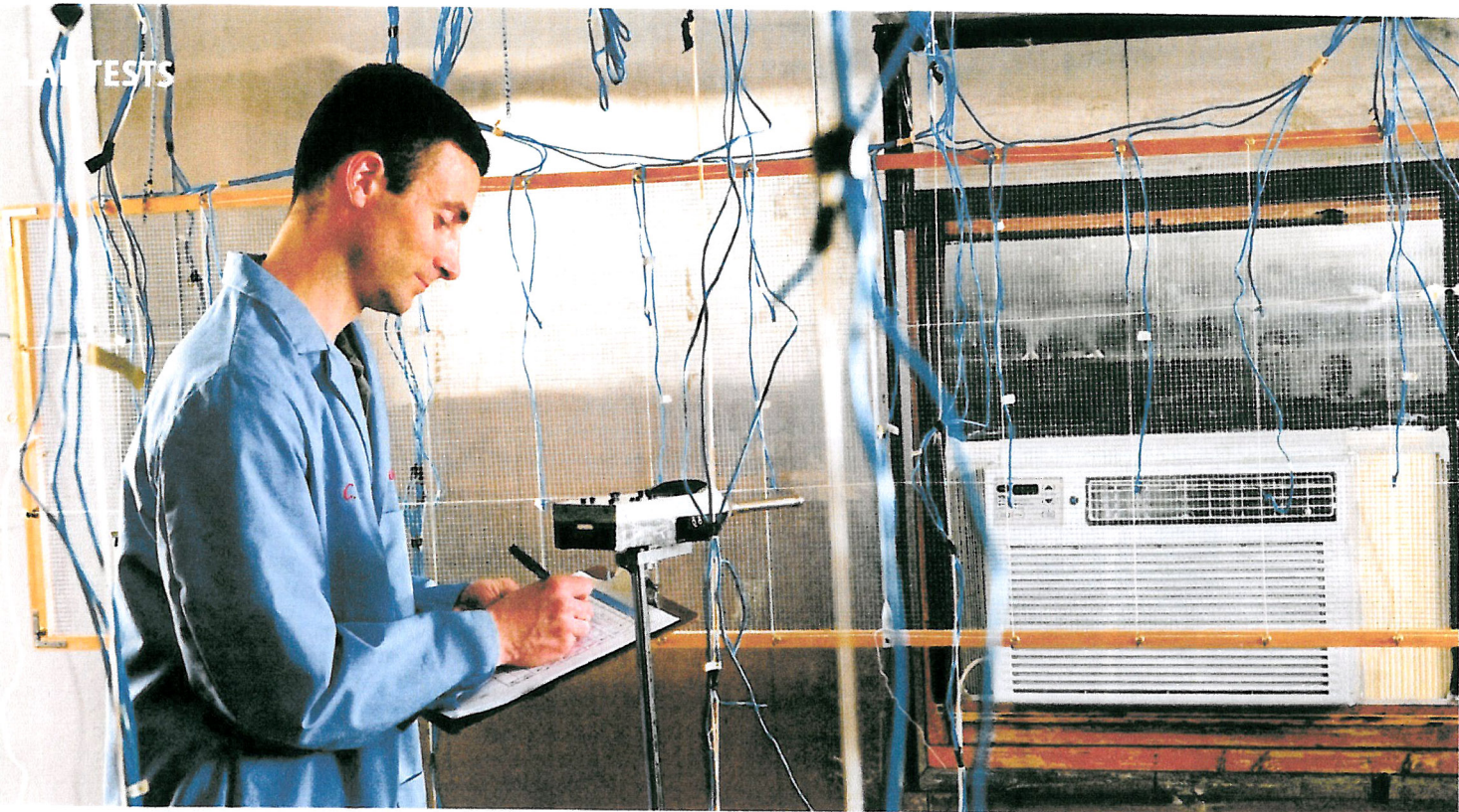
CHILLING CHAMBER Project leader Chris Regan checks readings in our temperature- and humidity-controlled air-conditioner room.
